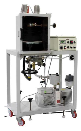
The resin degassing system is fitted with an Edwards E2M18 vacuum pump, complete with exhaust mist filter and inlet trap and solenoid operated air admittance valve.
