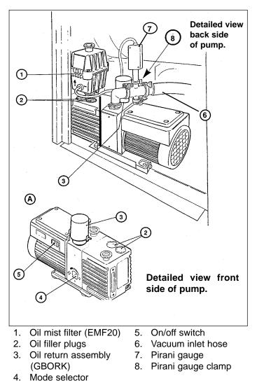
Figure 9. Vacuum pump components
