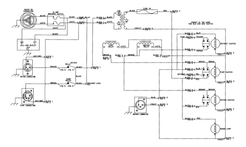
Figure 13 - SuperModulyo freeze dryer control module circuit diagram
