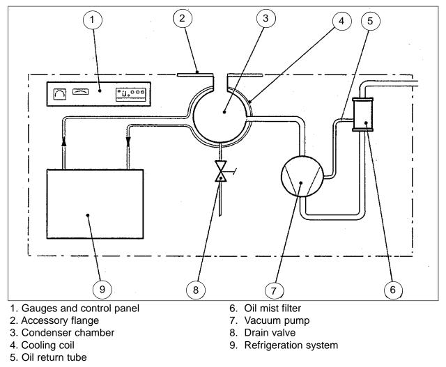
Figure 2. Schematic illustration of SuperModulyo freeze dryer components
