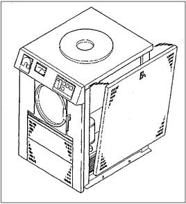
Figure 7 - Remove the side inspection panel
