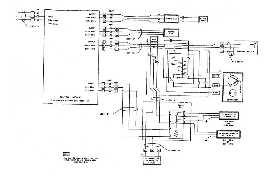
Figure 14 - SuperModulyo freeze dryer circuit diagram
