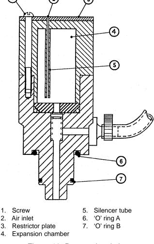
Figure 12. Part sectional view of the oil return assembly
