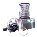
Add a drying accessory, such as the Acrylic Chamber and Tray Accessory, vacuum pump and optional, purpose-built SS trolley for a complete, freeze drying solution.
