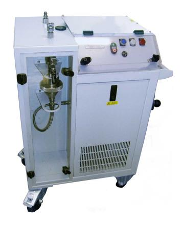
The front control panel comprises a flow controller / display, a pump on / off button, fault and power indicators, buzzer and mute control.
